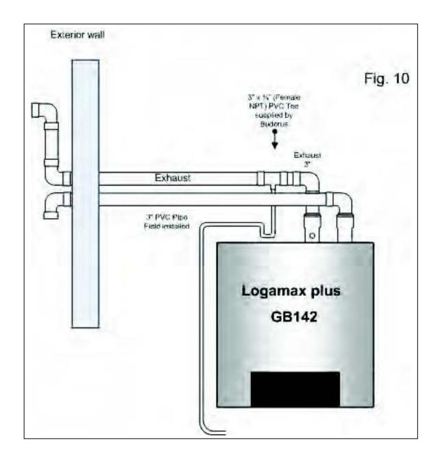
**Multiple Heater installation** – Terminate all exhaust vents at the same height and all combustion air inlets at the same height, while maintaining the minimum 12 inches vertical height clearance from between exhaust and combustion air inlet. Exhaust vent termination edge shall be at least 12 inches laterally from the edge of the air inlet pipe of an adjacent heater. The combustion air inlet is part of the direct vent system and not classified as a forced air inlet.
