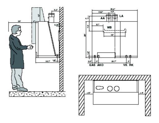
Fig. 2: Dimensions and Connections for GB142/45 and /60.
