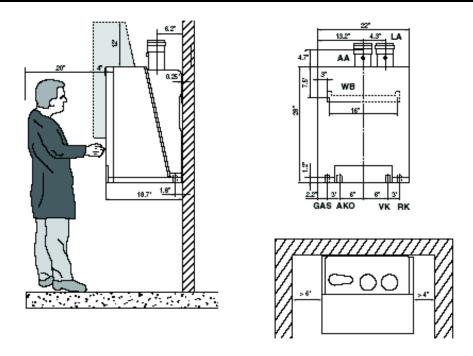
Fig. 1: Dimensions and Connections for GB142/24 and /30.
